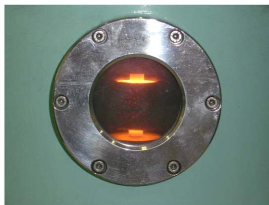
Fig. 1. (a) Experimental set-up of the spark plasma sintering system and (b) a photograph of a graphite mold and punches during sintering of an inert matrix fuel.
